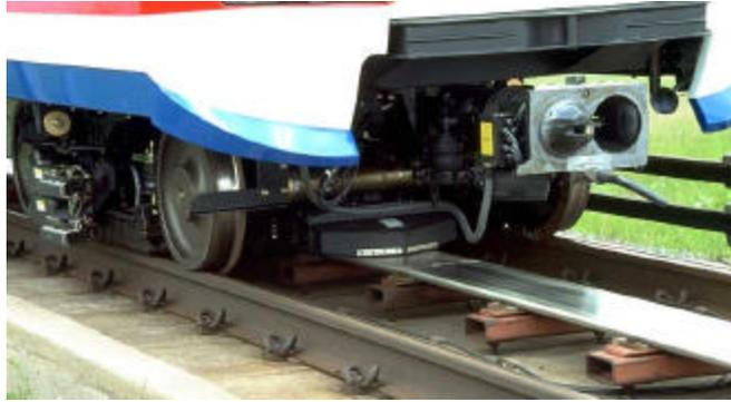
Figure 3.1-2 Vehicle guideway interface
